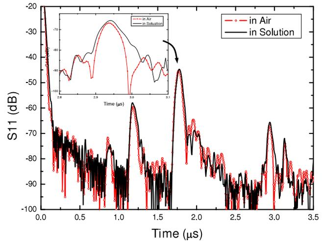
**Figure 10.** Comparison of the values of  $S_{11}$  measured in air and liquid solution.
