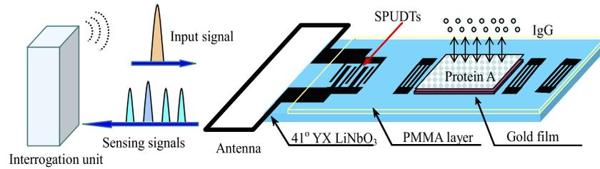
**Figure 1.** Schematic diagram of the developed Love wave mode biosensor system.
