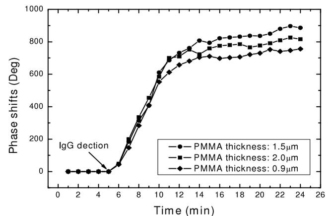
**Figure 12.** Comparison of sensor phase response depending on the PMMA waveguide layer thickness at the IgG concentration of 40 nM.
