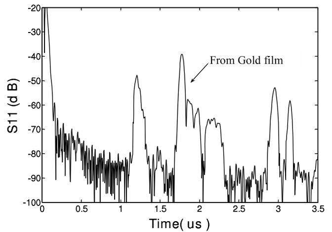
Figure 8. Measured reflection coefficient  $S_{11}$  of the Love wave device in the time domain in the case of no IgG binding.
