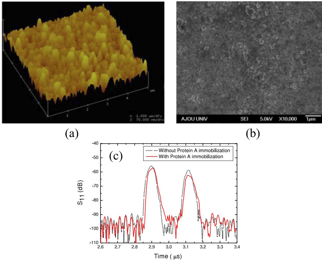
**Figure 11.** (a) AFM image of protein A surface, (b) SEM image of immobilized protein A molecules on the gold surface, and (c) the measured  $S_{11}$  in cases with and without protein A immobilization.
