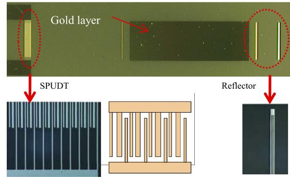
Figure 7. Optical microscope views of the fabricated devices.
