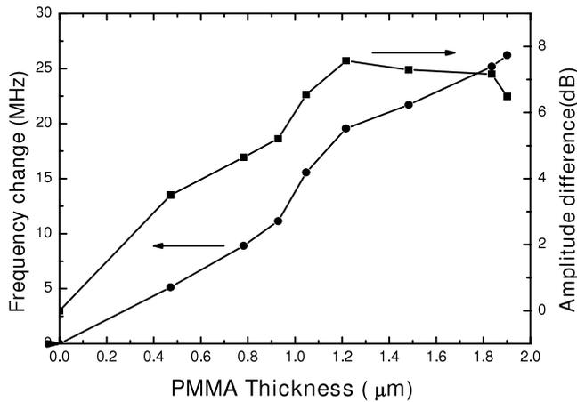
**Figure 9.** The changes of the resonance frequency and the amplitude of the reflection coefficient  $S_{11}$  as a function of PMMA thickness.
