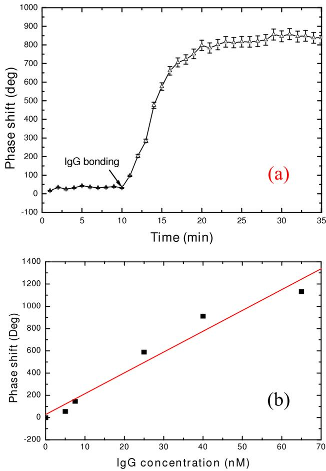
**Figure 13.** (a) Reproducibility results of the fabricated sensor in a constant 40 nM IgG solution, (b) phase response of the fabricated sensors in the IgG concentration range 0–65 nM.
