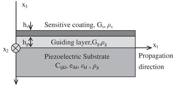
**Figure 2.** The coordinate system for the Love wave propagation analysis.
