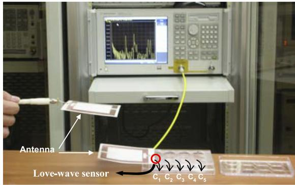
Figure 6. Wireless measurement setup of the biosensor system.
