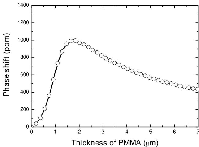
**Figure 4.** The phase shifts as a function of different PMMA thickness for the Love wave device with fractional thickness  $kh_s$  of 0.01.
