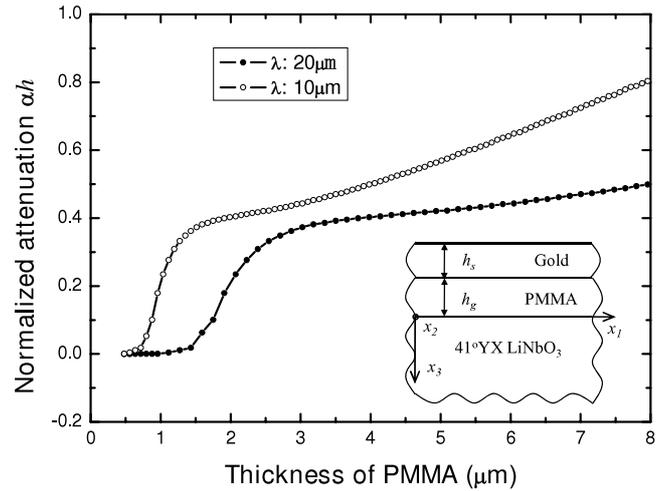
**Figure 3.** The attenuation coefficient versus PMMA guiding layer thickness as a function of different operation frequency.
