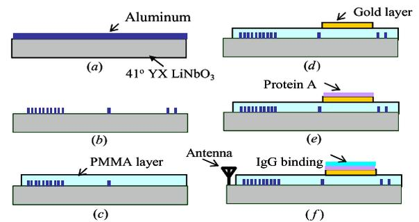
**Figure 5.** Fabrication procedure of a Love wave sensor. (a) Al deposition, (b) IDT and reflector pattern, (c) PMMA spin coating, (d) gold thermal deposition, (e) protein A coating, and (f) protein-IgG binding.
